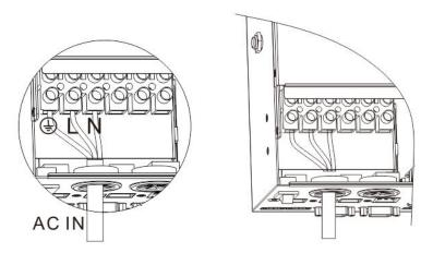
③ Correctly connect AC output wire in accordance with cable sequence and terminal position shown in the figure below. Please connect the ground wire at first, and then live wire and null wire. The ground wire is connected to the ground screw hold through O-type terminal.
