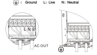
**Note:** The grounding wire shall be as thick as possible (cross-sectional area is not less than 4mm<sup>2</sup>). The grounding point shall be as close as possible to the solar storage inverter. The shorter the grounding wire, the better.
